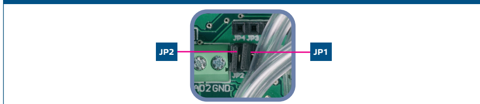
Fig. 5 Pull-up weerstand jumper
