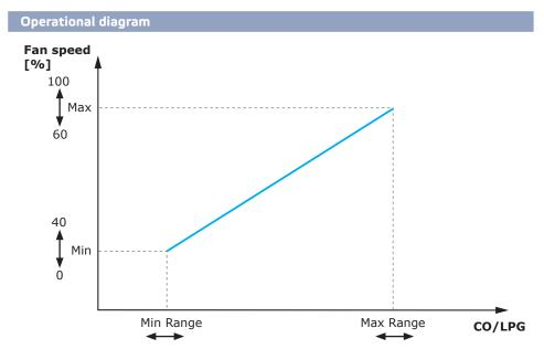
By default, the temperature, the relative humidity, the CO and the LPG sensors are active. It is possible to deactivate each one individually via Modbus. To regulate the fan speed based on CO and LPG only, deactivate the temperature and relative humidity sensors (and vice versa). When all sensors are active, the highest percentage value of all sensors will be used to regulate the fan speed.
