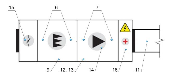
AHU overview with control and measuring equipment
