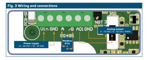
4. If your unit starts or terminates the network, make sure the NBT jumper is placed onto the pins as indicated in Examples 1 & 2 below. In all other cases, the jumper must not be connected. By default, the NBT jumper is disconnected - see Fig. 4 Network Bus Terminator resistance jumper.
