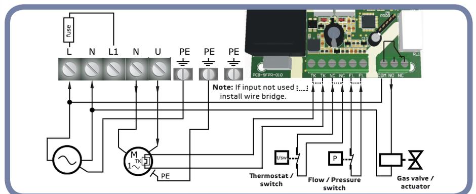
1c. Gas valve / actuator supplied from external 24 VDC supply.
