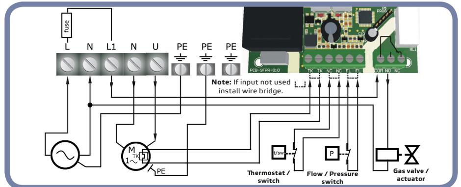
1b. 230 VAC gas valve / actuator supplied from L, N terminals without separate fuse protection (max. 6 A)
