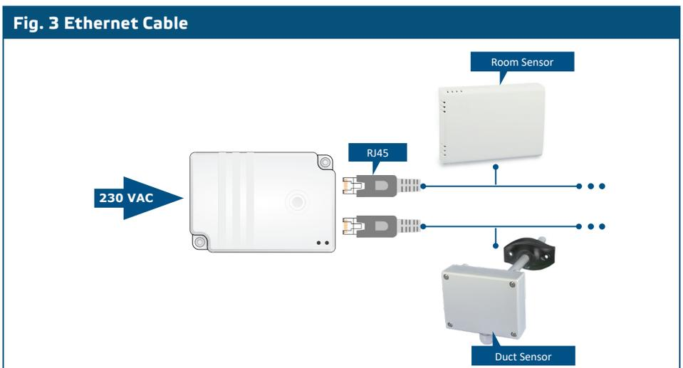
3. If the controller / sensor does not have an RJ45 socket, connect the wires of the cable as shown in **Fig. 4 Connecting cable** and do the wiring using the information from section **“Wiring and connections”** above .
