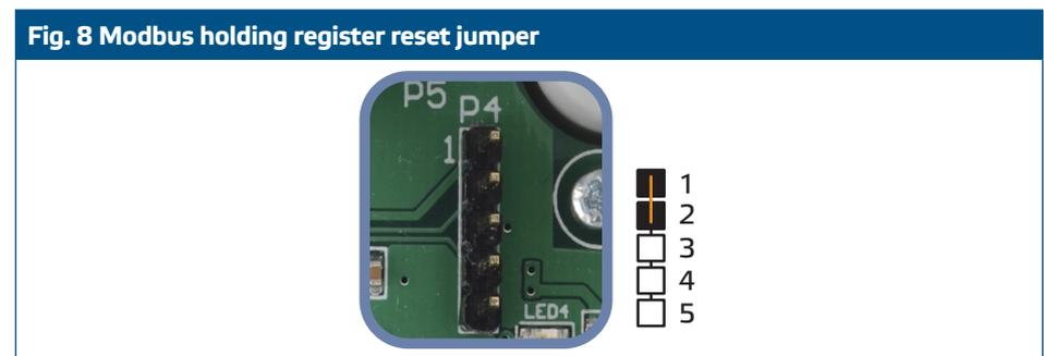
2. Modbus communication holding registers from 1 to 3 will be reset to the default values.
