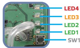
5. Sensor element failure indication:
