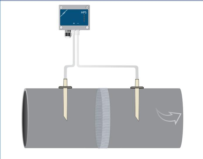
**Application 2: Measuring volume flow [m<sup>3</sup>/h] or air velocity [m/s] using PSET-PT**
