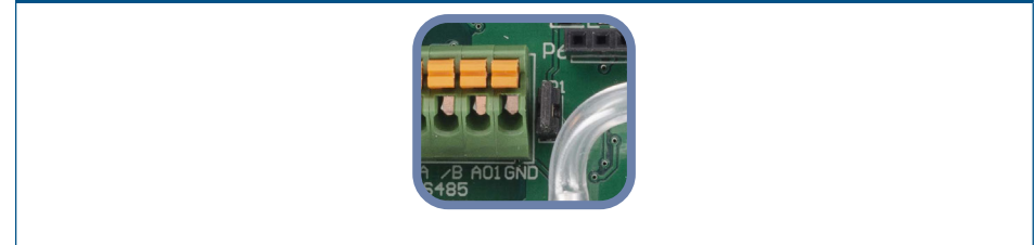
Fig. 5 Pull-up resistor jumper connected
