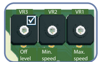
Fig. 8 Off level trimmer
