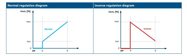
The **DRE** controller provides a normal / inverse regulation of the output signal (a percentage of the supply voltage).
