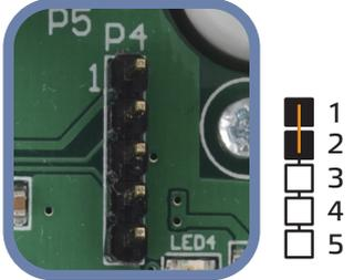
2. Modbus communication holding registers from 1 to 3 will be reset to the default values.
