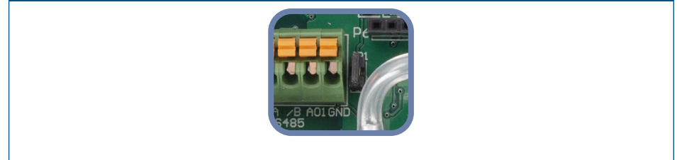
Fig. 5 Pull-up resistor jumper connected
