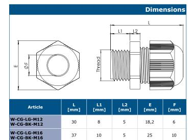
Note: The W-CN-XX-M12/M16/M20 cable gland nuts must be ordered separately.
