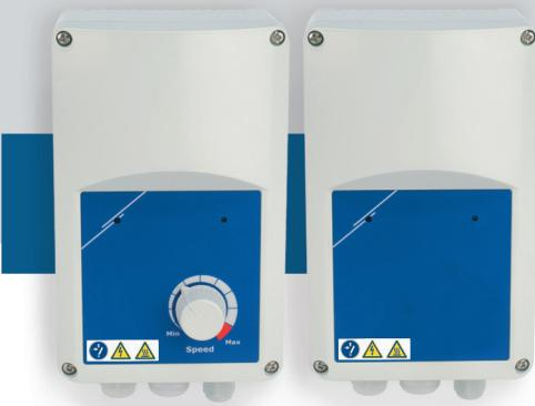
VFSC9 are electronic fan speed controllers for single phase induction motors (110–240 VAC / 50–60 Hz). They have a selectable analog input (0–10 VDC / 0–20 mA / PWM) and Modbus RTU communication. Compared to phase angle control (Triac fan speed controllers), the VFSC9 series generates an output signal with almost perfect sinusoidal shape, while the EMC pollution remains limited, the power factor exceeds 95 %.
