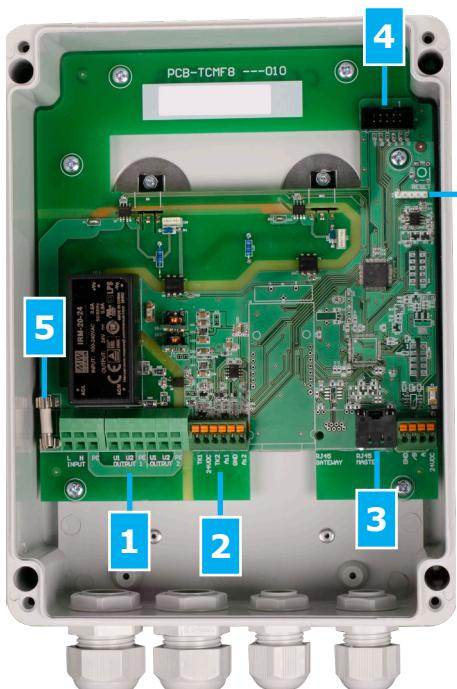
1 - Terminal block power supply and regulated outputs
