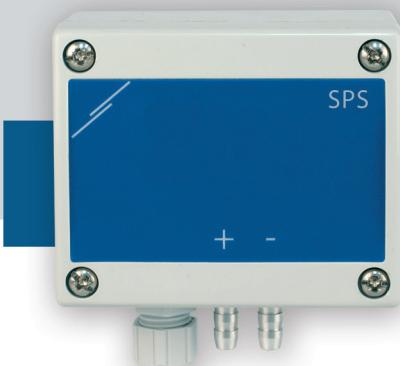
The SPSP differential pressure controllers control directly EC fans or drives. They are equipped with Modbus RTU communication and have an analog / digital output. The SPSP controllers feature integrated PI control, setpoint and K-factor setting. They are temperature compensated and provide a high degree of reliability and accuracy.
