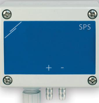
The SPS2 differential pressure controller directly controls EC fans, frequency inverters or other control units with two differential pressure setpoints (high/low or day/night mode option). It provides an analogue or digital output with integrated PI control and K-factor setting. You can switch between the setpoints by means of an external switch / contact or digitally. All system parameters are controllable via Modbus RTU communication.
