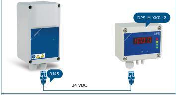
In this example, SEPS8 is connected to a differential pressure transmitter from the DPS-M-XKO -2 series via a cable with RJ45 connectors, which ensures both 24 VDC power supply and Modbus communication.
