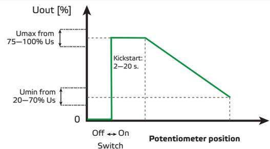
**Note:** By default, the desired fan speed or output value is set via the built-in potentiometer. It is possible to overrule the built-in potentiometer via Modbus RTU communication.
