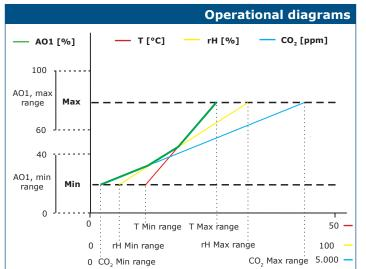
**Note:** The output changes automatically depending on the highest of the T, rH or  $CO_2$  values, i.e. the highest of the three output values controls the output. See the green line in the operational diagram above. One or multiple sensors can be deactivated. E.g. it is also possible to control the output based on the measured  $CO_2$  value only.
