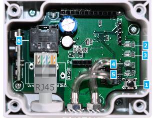
1 - Sensor calibration and Modbus register reset tact switch (SW1)
