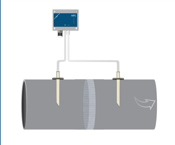
**Application 2:** Measuring supplied air volume [m<sup>3</sup>/h] or airflow velocity [m/s] using PSET-PT
