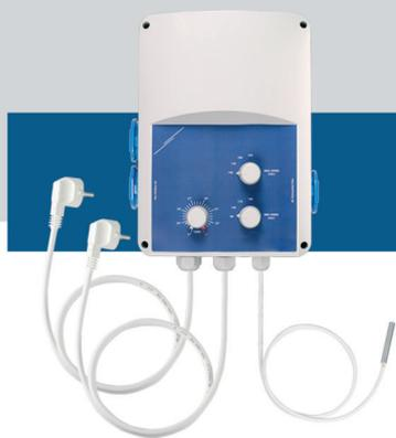
The GTTE1 series of transformer fan speed controllers regulate the rotational speed of single-phase voltage controllable motors by varying the output voltage according to a measured temperature. They are equipped with auto-transformer(s) and control the speed of the supply and extraction fan automatically in five steps according to the temperature input of the integrated flying lead sensor. An electric heater can be controlled (ON/OFF) via the extra output.
