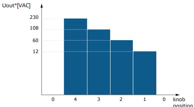
\* These are average output voltage values. Regulated output voltage depends on fan/motor characteristics of connected load ( $\cos \varphi$ ).
