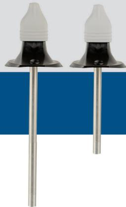
The DTS-L series are digital temperature sensors powered over Modbus with 3,3 VDC via an RJ12 connector. They are intended for duct channels and are compatible with various temperature control systems. The sensor element is placed in a stainless steel tube of different length - 85 or 165 mm, which simplifies the cleaning of the duct system.
