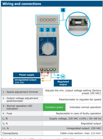
**Note:** To disable the OFF position, connect the 230 VAC supply voltage to the unregulated output (L1). In this case, do not connect the power supply to L. Set the minimum motor voltage according to the application requirements and motor specifications.
