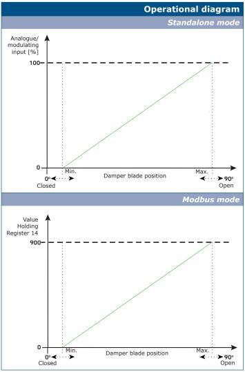
Attention! The minimum open and the maximum closed positions of the damper depend on the values set in Modbus Holding registers 17 and 18.
