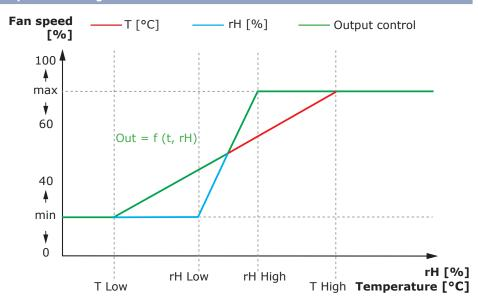
By default, both the temperature and the relative humidity sensor are active. It is possible to deactivate one of both. To regulate fan speed based on temperature, deactivate the relative humidity sensor and vice versa. When both sensors are active, the highest percentage value of both sensors will be used to regulate fan speed.
